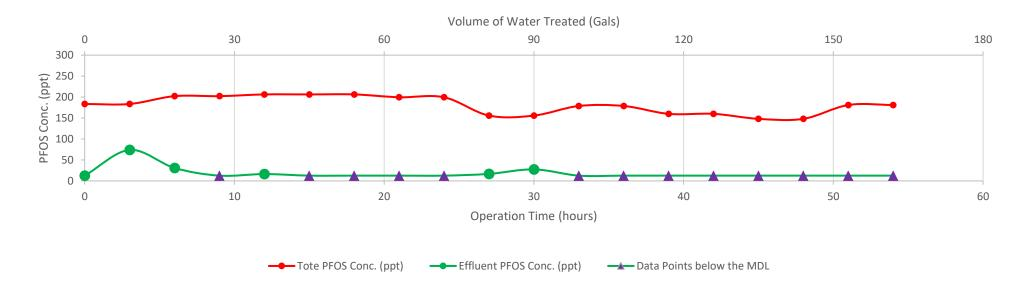
Results from our bench scale reactor have shown between 96% - 100% removal of PFOS after one treatment
